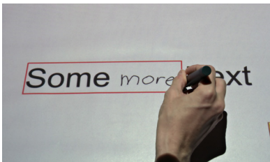
Figure 4: In situ text insertion with handwritten content. The right part of the string is gradually shifted as the user writes
